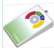
**Dimensions** 21.5 x 14 x 2.5/4.5cm 5cm cursor control ring Wired USB Connection For Windows & Mac 2 Switch Ports Double Click & **Drag Lock Function**
